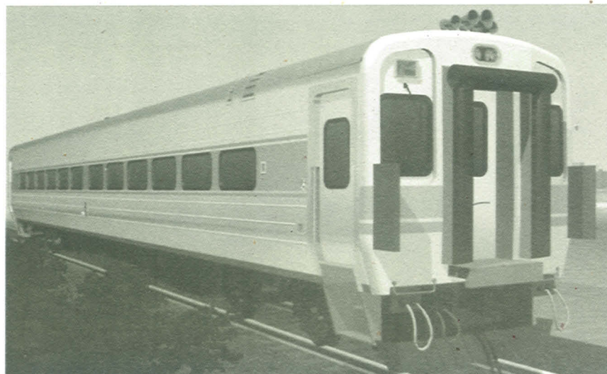
Nippon Sharyo's self-propelled diesel rail car seats 87 passengers and is designed for inter-city travel in the U.S.
